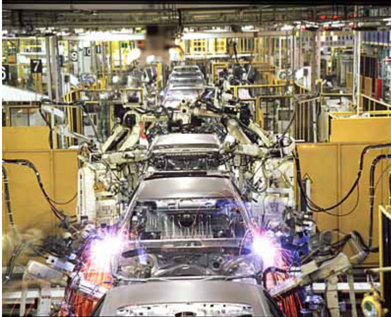
Figure 7: Welding robots at a Toyota automobile factory.
