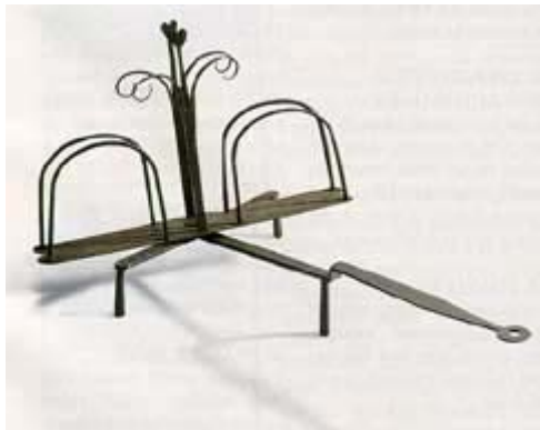
Figure 8: Hearth Toaster from the Walter Himmelreich collection, Pennsylvania, c. 1800. Bread was placed between the arches; when one side was browned, the toaster was rotated to brown the other side. Photo and caption from the Cyber Toaster Museum.
