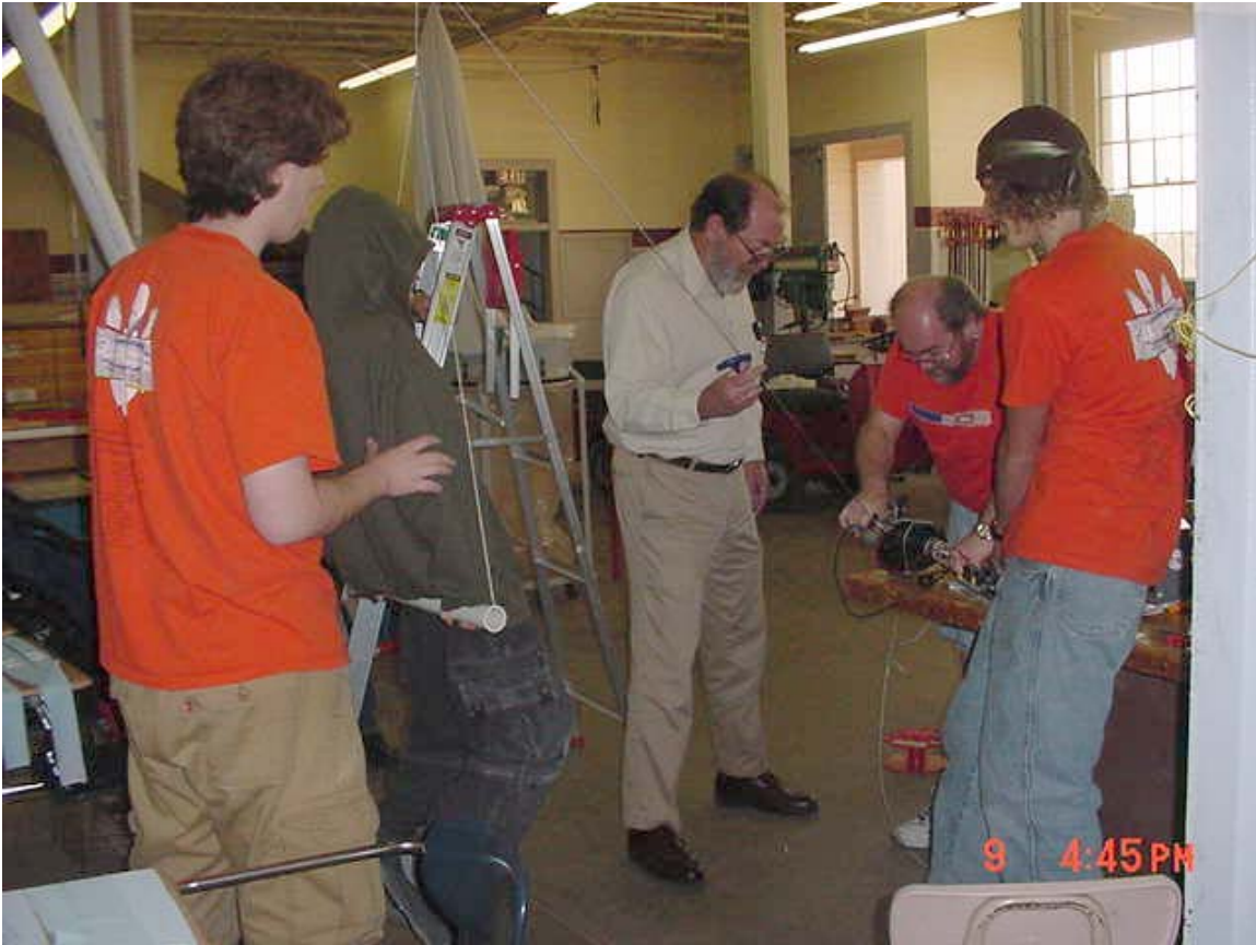
Figure 22: The winch assembly is tested to make sure it has enough force to lift the robot. A student on a swing acts as our weight.
